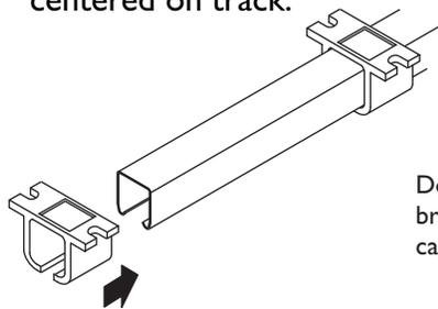
Do not install end brackets with end caps at this time.
