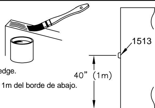
**8** Fasten 1513 Bumper on back edge of door 40" (1m) from bottom edge.
