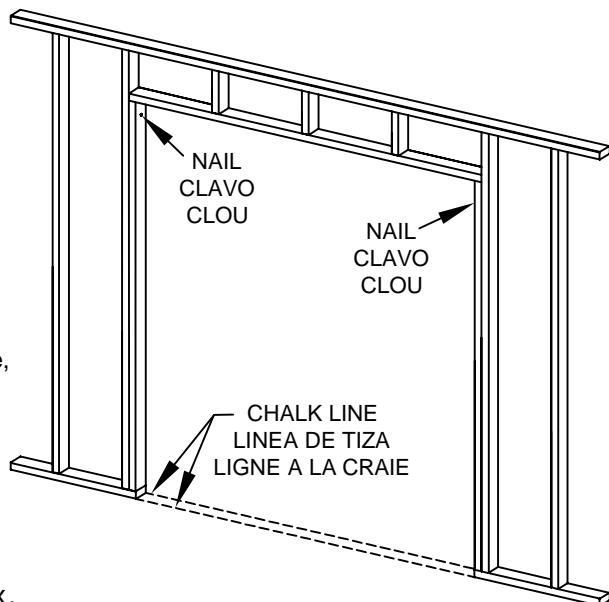
**4** Slip slots in Frame Header End Plates over nails in rough studs.
