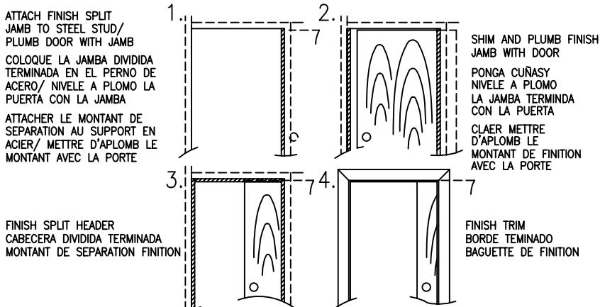
Fasten 1550 Guides on finished split jambs at door bottom so door is held in center of opening.
